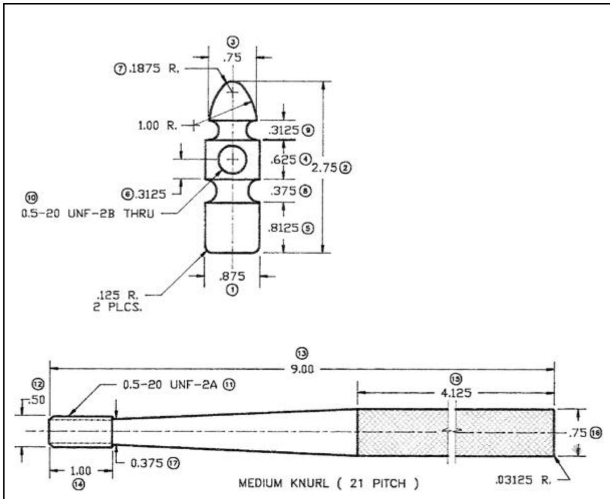
Figure 3: Hammer Parts: Head and Handle
