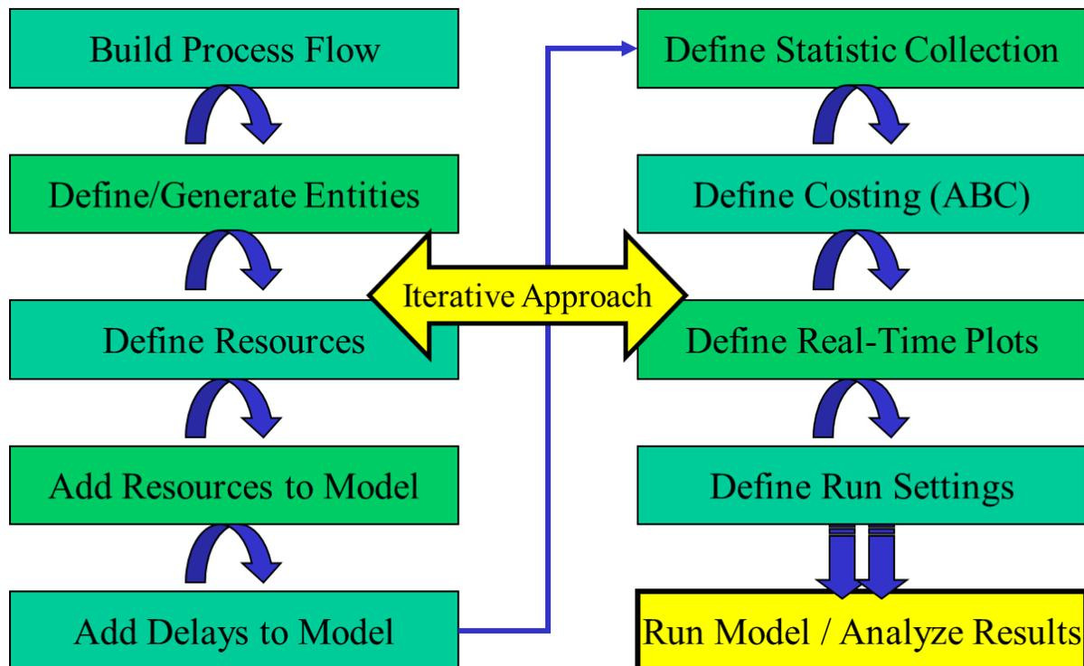
Figure 2. Steps to Simulation in SIMPROCESS (Courtesy of CACI, 2015)
