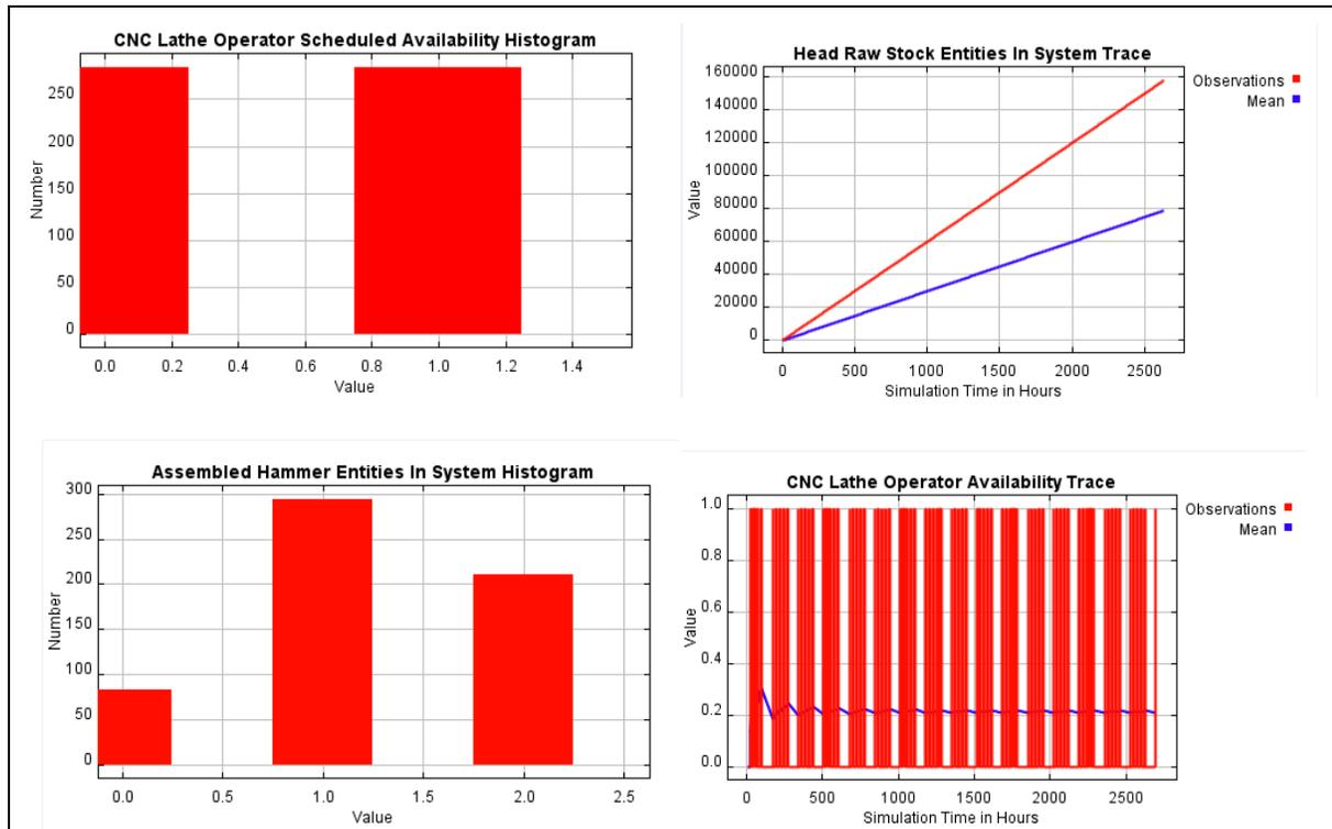
Figure 14: Real-Time Plots of CNC Operator and Some Entities
