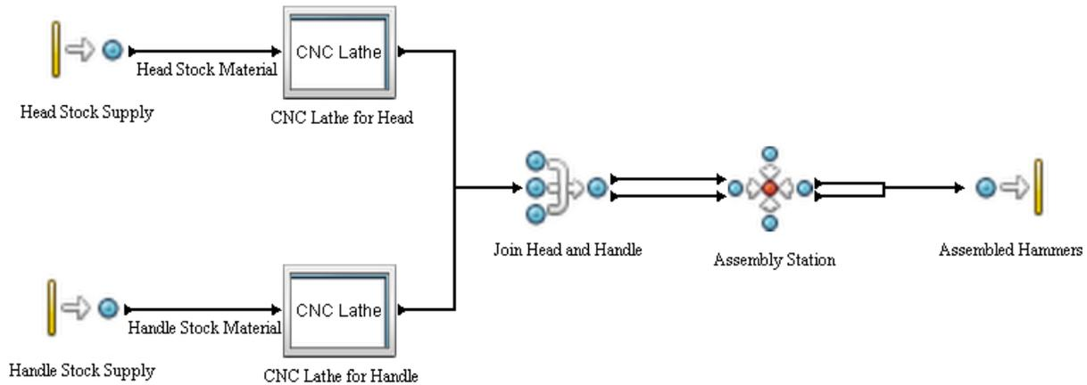
Figure 5: Flow Layout of the Hammer production Process
